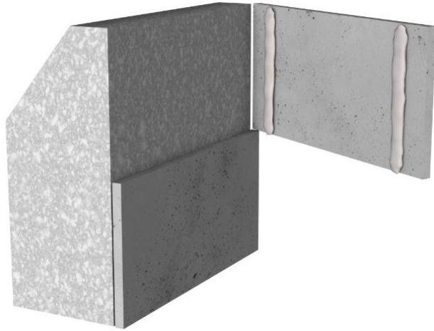
Figure 9. Gluing with dispersion glue
